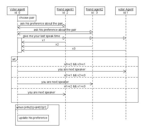
Fig. 4: UML sequence diagram representing communication between agent with Need to talk function.
