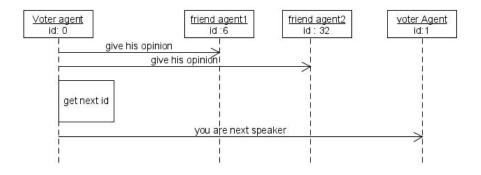
Fig. 1: UML sequence diagram representing communication between agent with round robin function.
