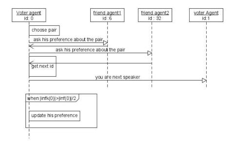
Fig. 3: UML sequence diagram representing communication between agent with round robin function.
