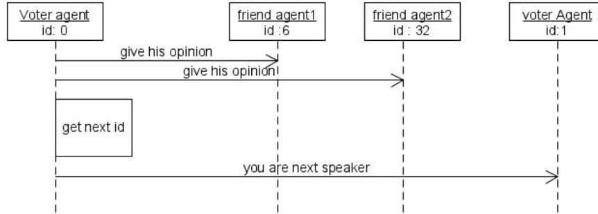
Fig. 1: UML sequence diagram representing communication between agent with round robin function.
