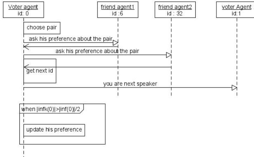
Fig. 3: UML sequence diagram representing communication between agent with round robin function.
