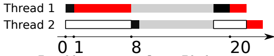
Figure 2: Possible execution flow. Black areas represent execution without locks, red areas - execution within a critical section, grey areas - sleeping, white areas - waiting for processor time.
