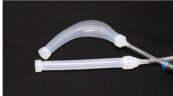
Fig. 1: 3D printed Soft Pneumatic Actuator using our LLS fabrication technique. (Bottom) The actuator shape is unaltered when non-pressurized. (Top) The actuator bends when pressurized.
