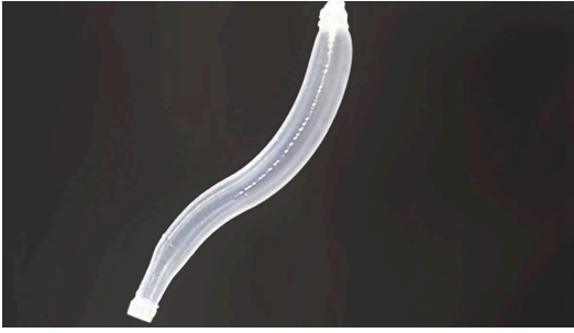
Fig. 7: Example of multiple bending SPAs made with the LLS method. The SPA nozzle diameter is T = 0.86\text{mm} , and each side of the actuator has a different layer height value. These values are swapped at half of the actuator, which results in a two-directional bending.
