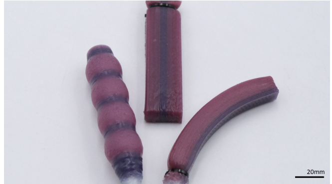
Fig. 1: SPAs printed with silicone dynamic mix ratio modification layer-by-layer. Left) Printed standing resulting in linear extension when inflated (currently inflated). Right) Printed flat resulting in angular deformation when inflated (currently inflated). Center) Multi-channel actuators printed flat, resulting in increased bending control (not inflated).
