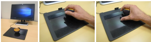
Figure 7. Overview of the RPM input apparatus (left): rolling RPM (centre) and tapping on the tablet to validate (right).
