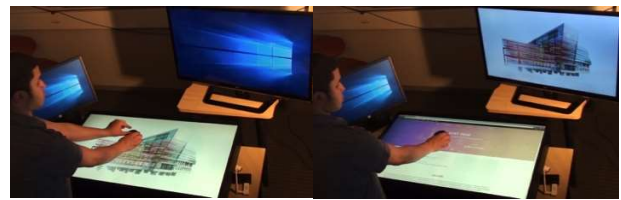
Figure 5: A Translation + Spread gesture sends the tabletop content (left) to a secondary display (right).
