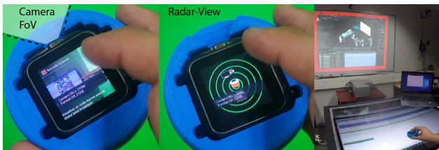
Figure 4: TDome's on-board camera detects displays (left) and creates a radar-view of the spatial layout (center). Then the user can select a display by Rolling + Tapping towards it (right).
