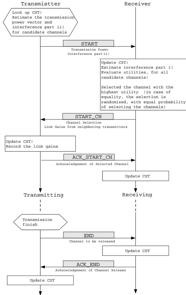
Fig. 1.2. Handshaking Process for the Signaling Packet Exchange
