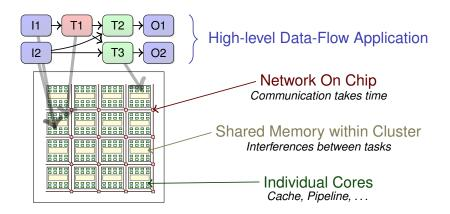
→ Implementation of a dataflow application on a many-core → with intra-cluster communications
