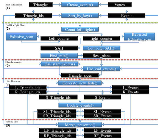
Figure 1: GPU large node processing implementation details, step by step. Blue cells for CUDA kernels, black cells for data. L=left, R=right, S=shared, F=final.
