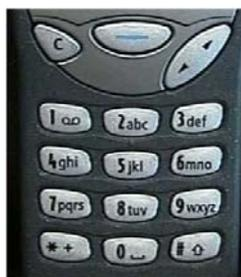
**Figure 1.** The keypad layout on a Nokia 3210.
