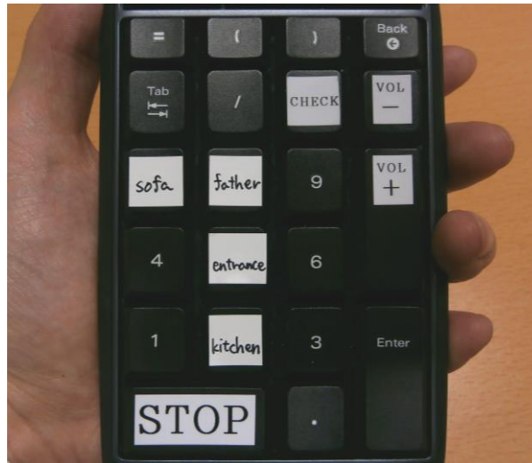
Fig. 5. Labeling by Physical Labels. The user attaches physical labels on a remote control to name locations. The labels of the targets can be static like “kitchen” and “entrance,” semi-static like “sofa,” or dynamic like “father.”
