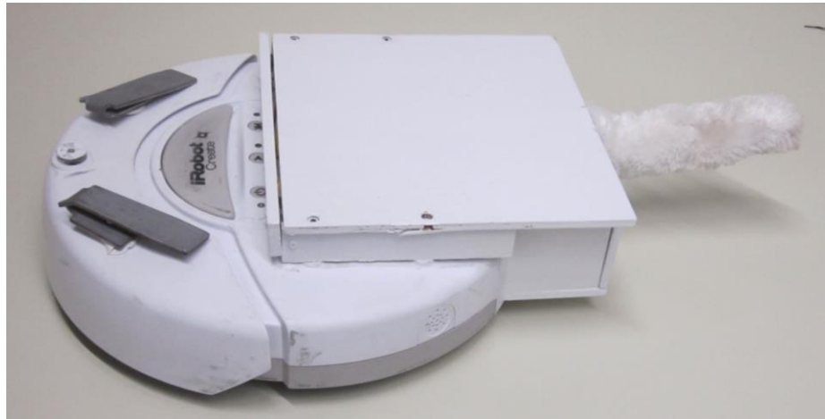
Fig. 2. An iRobot Create with our dog-tail attached.
