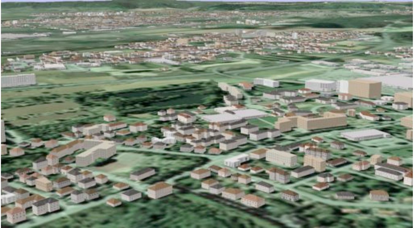
Figure 15: Urban area made of 17 362 buildings, the building generation took 7mn and 55sec, 920 182 faces were generated.
