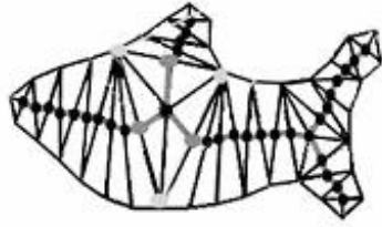
Figure 6: Computing the radius in isolation and the blobbiness for the center point. The light gray points participate in radius in isolation computing. The dark gray points contribute to the blobbiness value.
