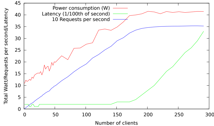
Figure 3: Zoom on Intel I7 serving a web workload. Scales are adapted to be visible. Points are average value of 10 experiments.
