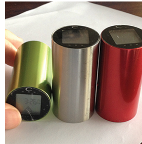
Air quality low-cost sensor Tiny, low cost & High spatial/temporal granularity Low installation & operational cost Less accurate Regular calibration
