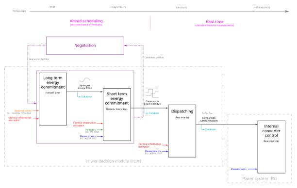
Figure 2 : different optimization levels of the power decision module
