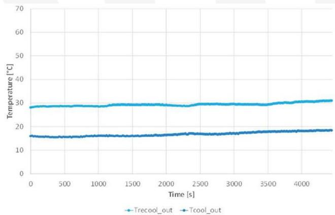
Fig. 10. Fluid temperatures measured at the adsorption machine external circuits: re-cooling (cyan) and cooling (blue).
