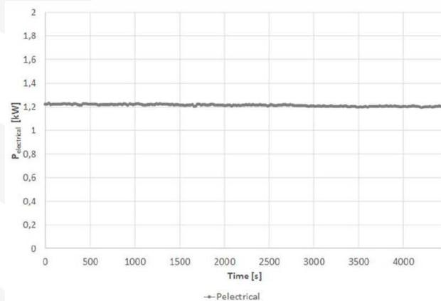
Fig. 7. Electrical power at the output of the PVT array.
