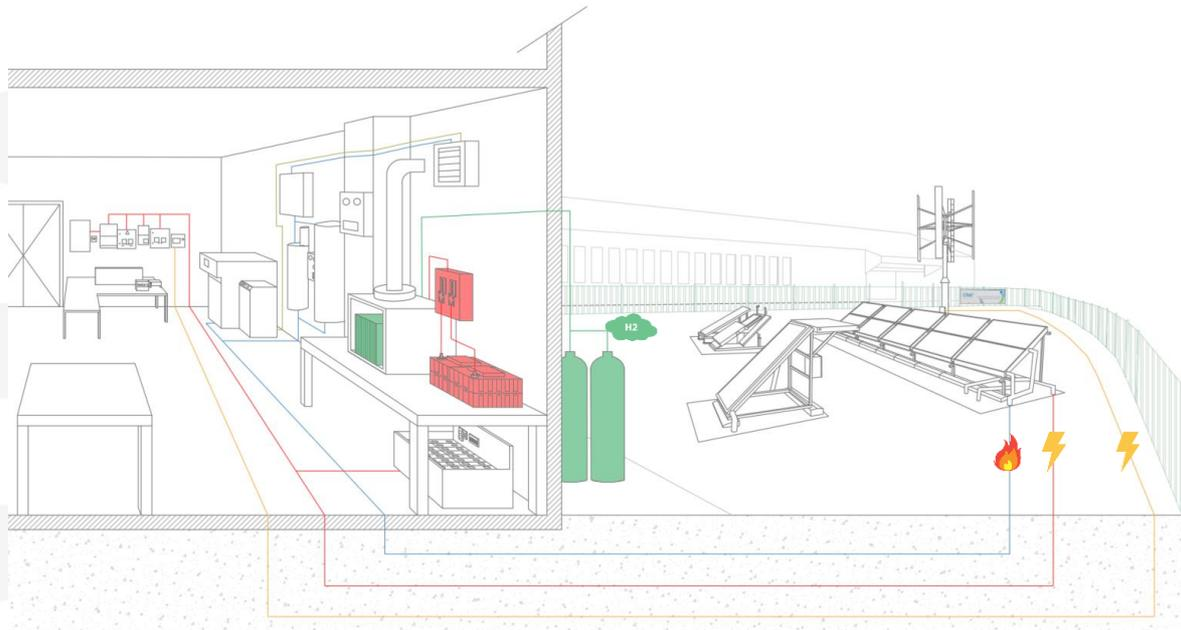
Fig. 4. Hydrogen system.
