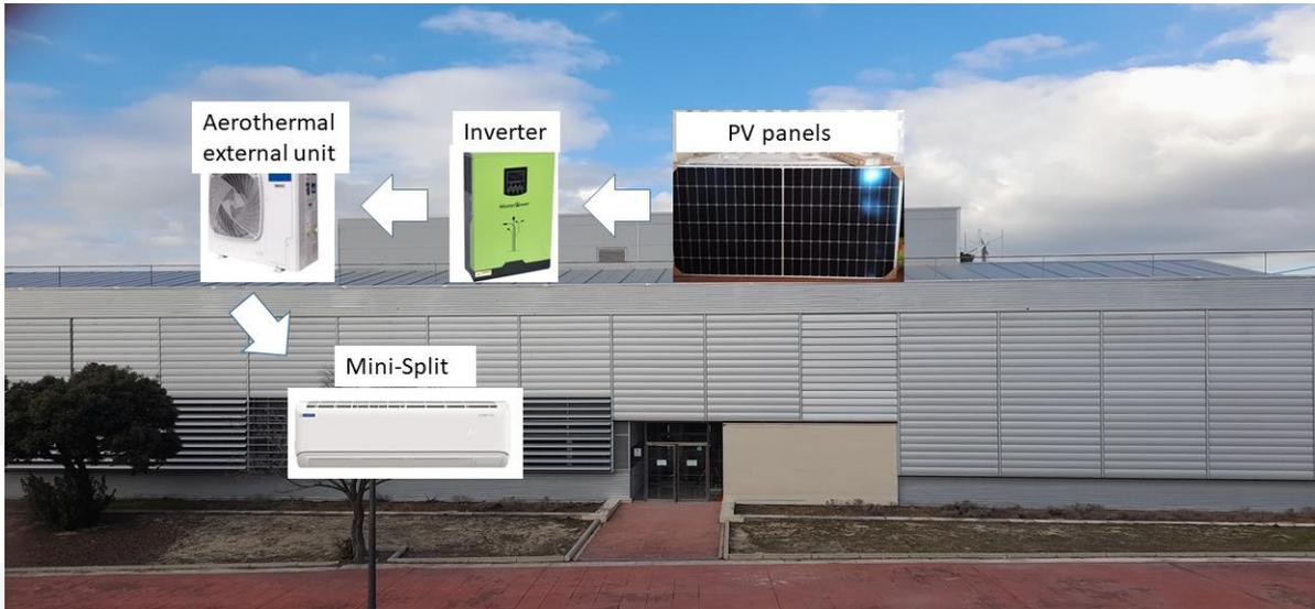
Fig. 18. Architecture of the PV-powered aerothermal source for HVAC of the IoT laboratory.
