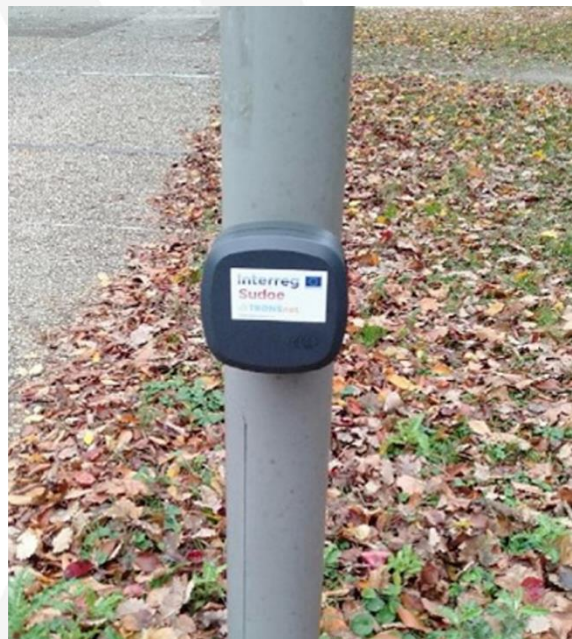
Photo 3. Pyro-Box Evo: pedestrian counter
