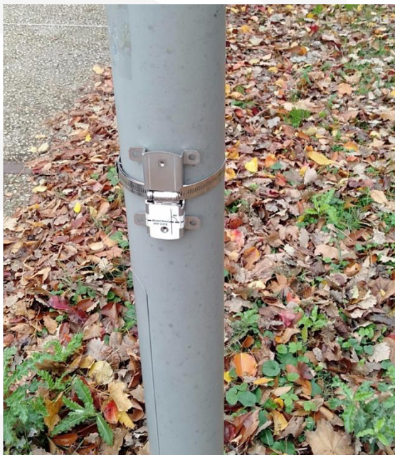
Photo 3. Pyro-Box Evo: pedestrian counter
