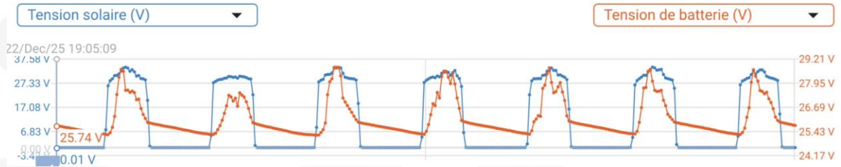
Figure 9. 7 days measurements of the solar generator voltage (blue) and battery voltage (orange).
