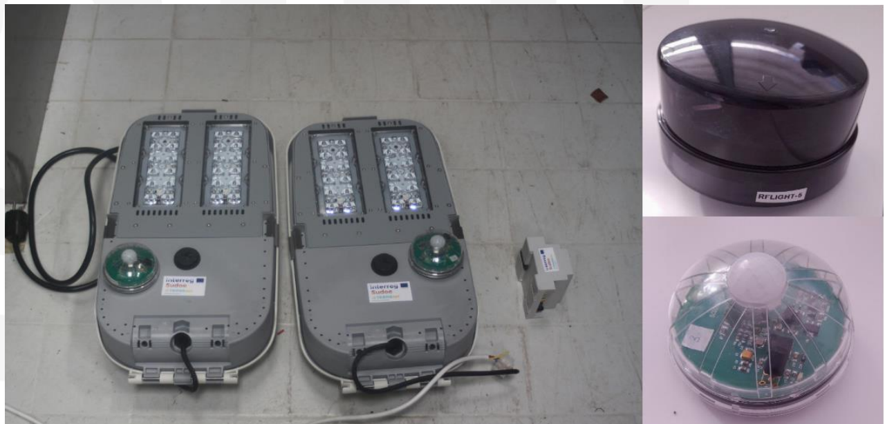
Figure 4 : The BatStreetLight fixtures received in Toulouse with the BSL communication device (right upper part) and IoT Presence Sensors (right lower part)
