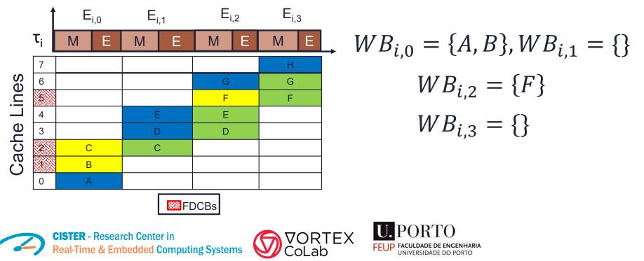
• Cache write-backs during the execution of a scheduling interval E\_{i,j} depend on the ECBs of that scheduling interval and FDCBs of all tasks in hep(i) and lp(i)
