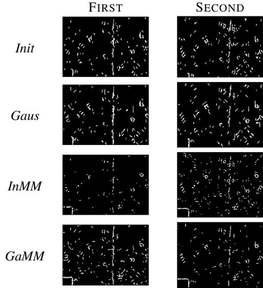
Figure 3: Crack detection – Examples of the results of the four variants on one image, see image with 10° and *ambient* light in Figure 2. White pixels correspond to pixels considered as a crack. The *Init* and *Gaus* methods show a quite dense detection, with a lot of false detections, whereas, the two others are more sparse but with less false detections. A quantitative analysis is given in section 4. For each variant, it illustrates how the results are complementary.
