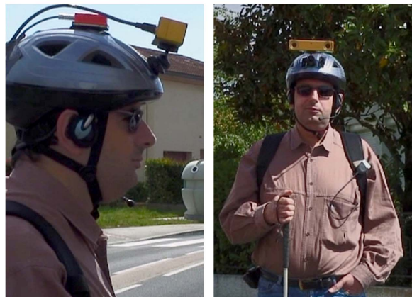
Fig. 2. NAVIG prototype including a GPS receiver, a stereoscopic camera and a head motion tracking device mounted on a helmet. Microphone and headphones were added for speech and audio
