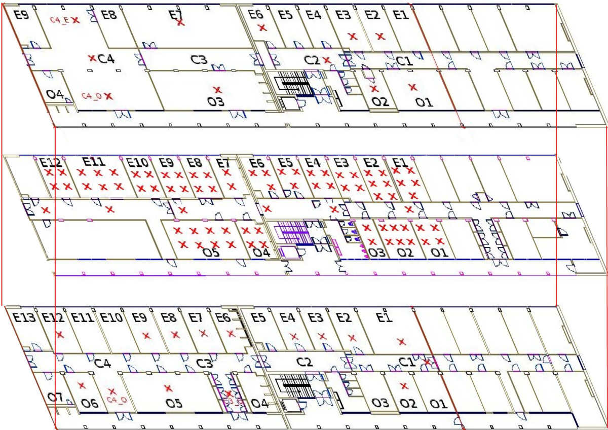
Figure 4: Experimental configuration. The test building is made of three floors. The source is located in room E7 at intermediate level. Measurement points are indicated by red crosses.
