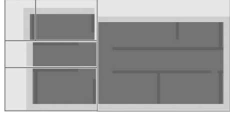
Fig. 7. The irregular descendant tree building: the head MR-node is cut along the best discontinuity and so on for its children. The process is herein shown for the head node and "top and left" children recursively.
