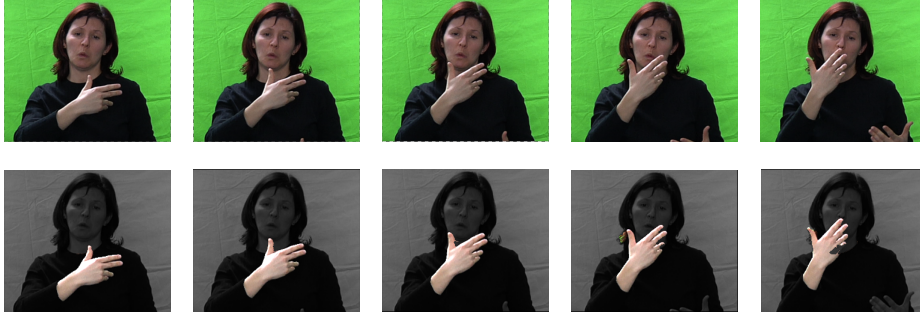
Fig. 4: First row shows five consecutive frames in a sequence with hand over face occlusion. The second row shows the segmentation result. Pixels in dark gray or in black have been classified as belonging to the non hand class, otherwise they are shown in their natural colour.
